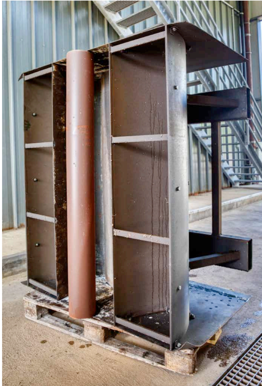
Reusable steel formwork for the production of Sorel concrete prefabricated parts
