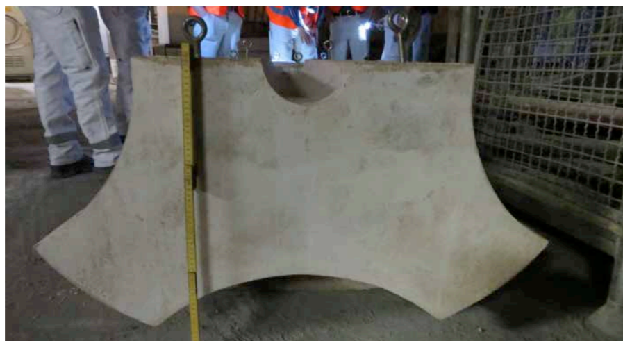
A prefabricated part made from Sorel concrete
