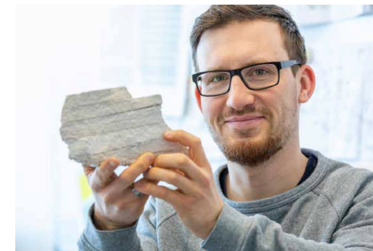
Another sample in the hands of Marcus Tresper. It shows the layered structure of the individual concreted batches.
