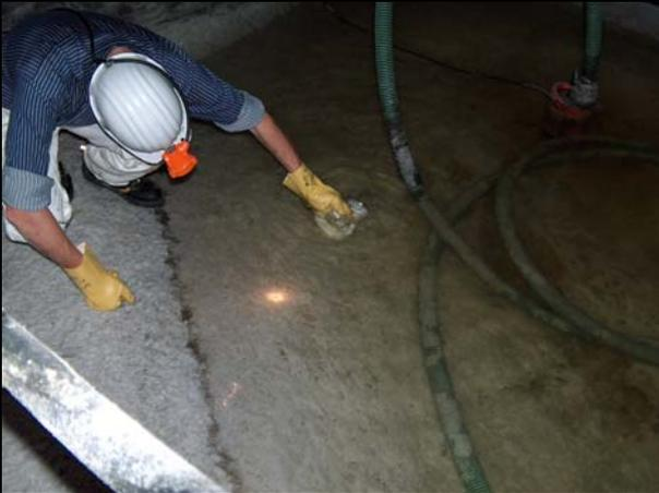
**Photo 32:** Feststoffprobe MP 38-F1 (Bodensatz/
